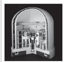
The first Pressurized Water Reactor built in Britain is based on a US design and produces 1250 MW of carbon-free electricity. The fuel is uranium dioxide, supported in the reactor pressure vessel, which is filled with water under high pressure. Water is pumped through the reactor to carry heat away from the fuel. The hot water passes through a heat exchanger that heats a second supply of water. The secondary water boils, and the resulting steam drive the electric generators.
